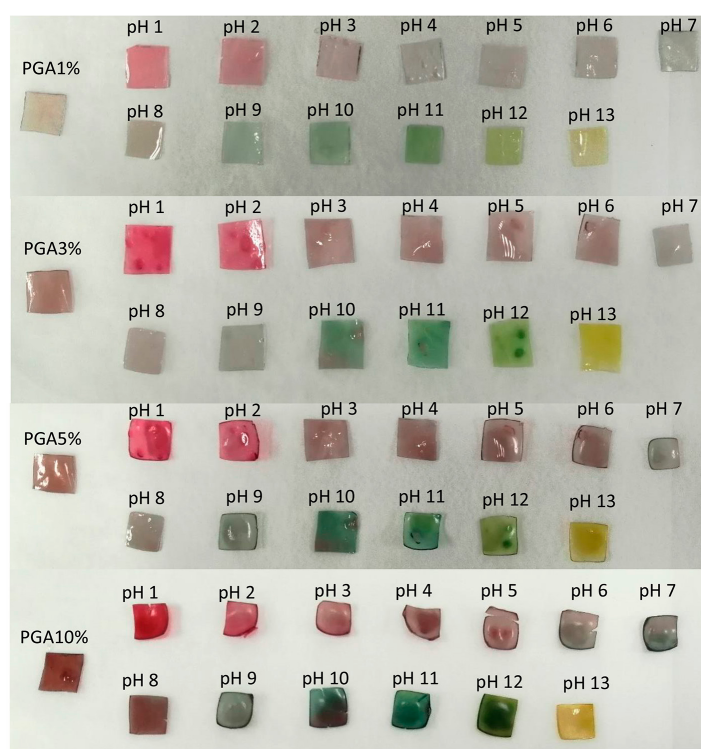
Figure 6. Color response images of films from pH 1 to 13.
